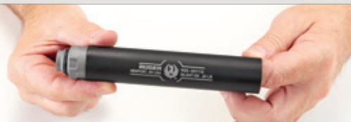
Slide the Entire Stack of Baffles Out of the Rear of the Suppressor Tube
